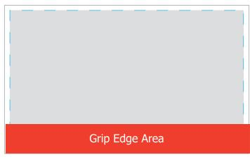
The area shown in grey is the area that can be Foil Stamped. We require a 10mm space at the bottom or the top of the card for the hot foil machine to grip the card.
